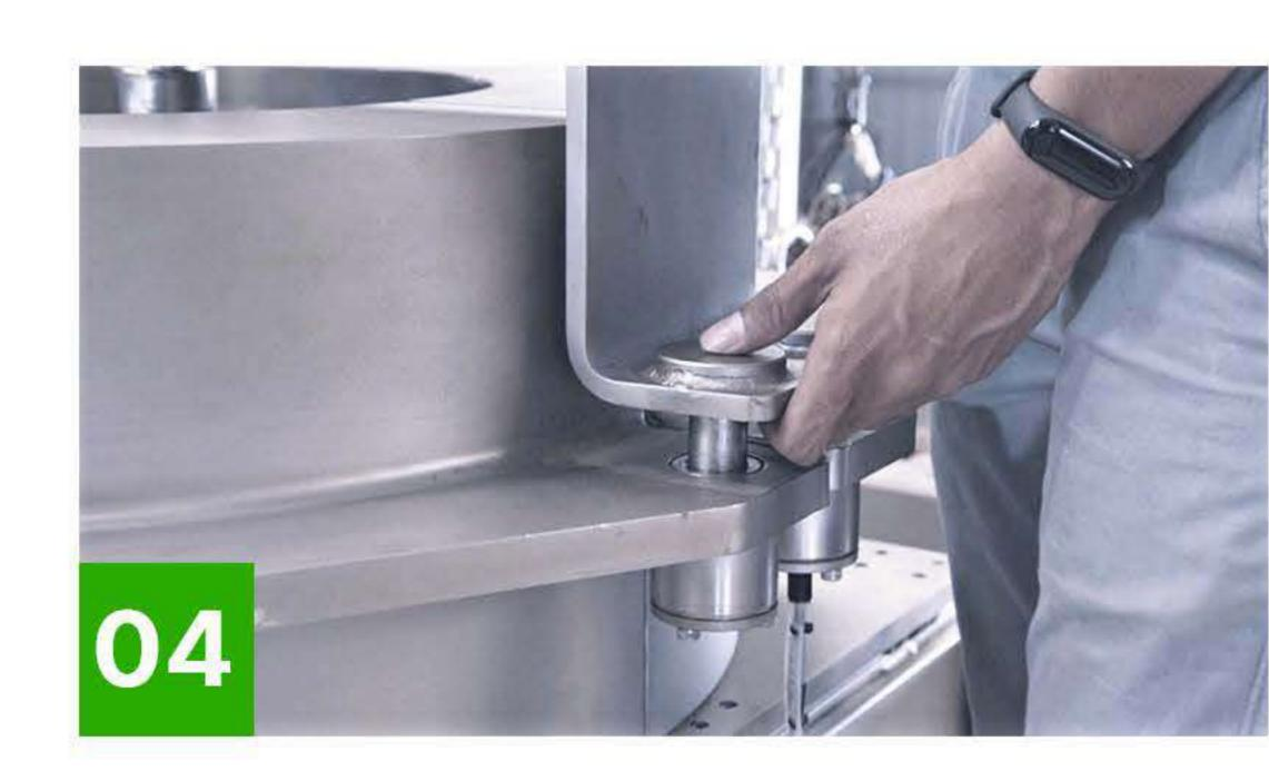
Unique Extractor Closure Design for rapid batch changeovers with minimal interruption
